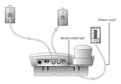
Fit the power cord behind the strain relief tab. Then plug the smaller end into the power jack on the back of the system.
